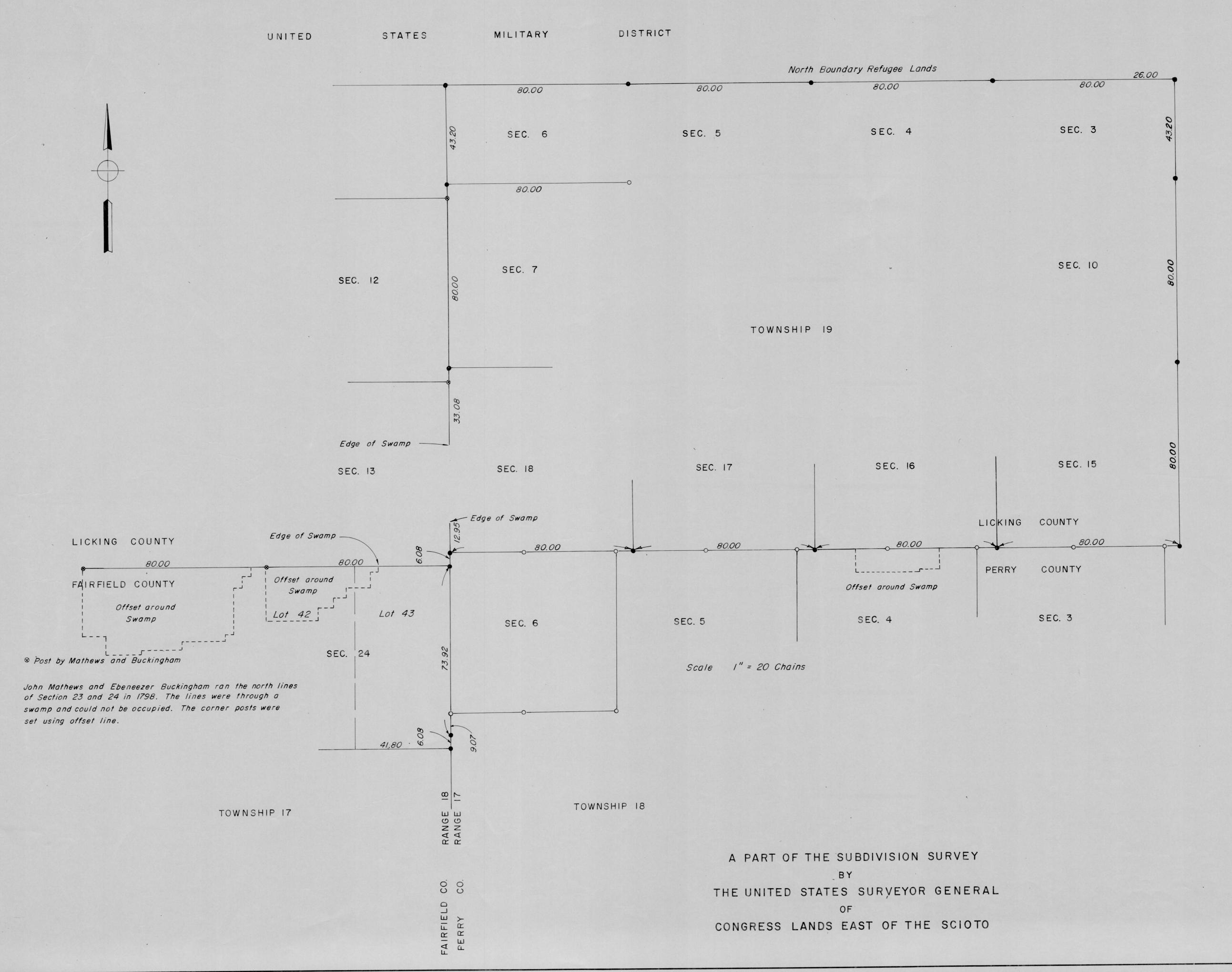
John Mathews began at the southwest corner of Section 18 and traversed to the southeast corner of Section 15, to the northeast corner of Section 3, to the northwest corner of Section 6, and through the northwest corner of Section 18 to the edge of the swamp in 1798.
